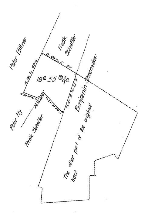
Draft of a tract of land situate in Lowhill township, Lehigh County, containing 1895. 55 13 and allowance of six per cent for roads, &c., surveyed for Fredk. Shaffer the 12th day of June A. D. 1872, being a part of a larger tract of 102 95 136 B &c. originally surreyed to Henry Kretlow, by Appl. No. 1390, dated 10th April 1766. Geo. Blank, C.S.
